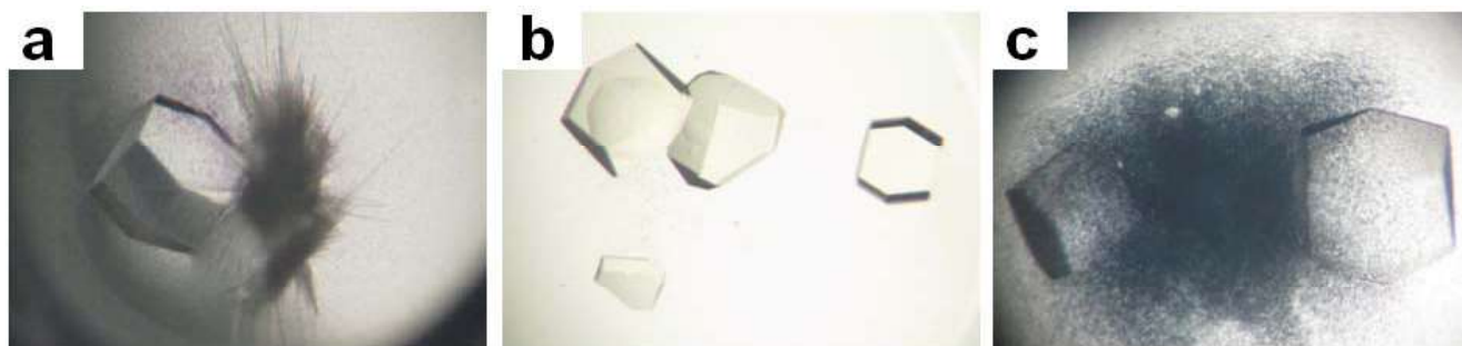
Figure S5. Photos of the crystals grown from lysozyme and preformed gold nanoparticles of different sizes. (a) 13 nm gold nanoparticles stabilized by sodium citrate (17 nM), (b) 5 nm gold nanoparticles stabilized by sodium citrate (82 nM), and (c) \sim 1 nm \text{Au}_{102}(\text{para-mercaptobenzoic acid})_{44} (1 mM).
